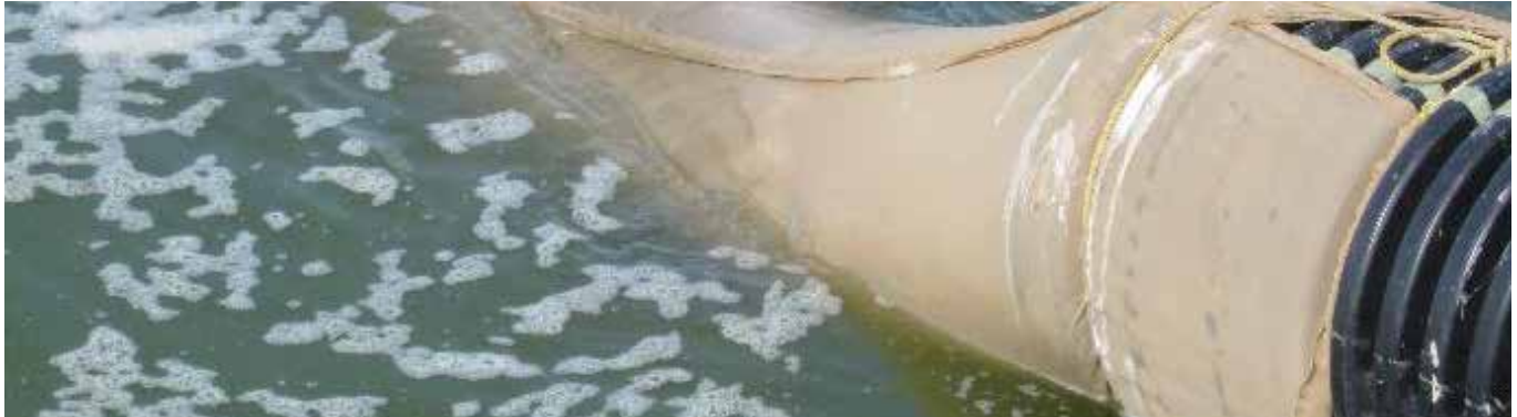
The use of smaller micron (<280) bag filters can keep many vectors out of ponds
