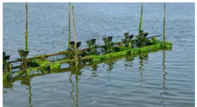
Figure 4: Large amounts of filamentous blue green algae on paddlewheels
